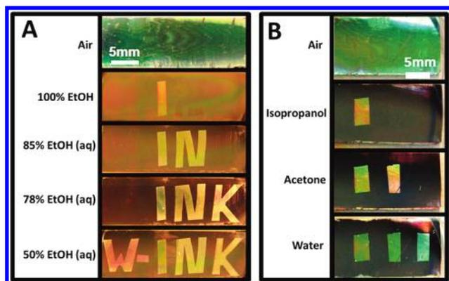
**Figure 2.** (A) Optical images of an IOF in which the word “W-INK” is encoded via the surface chemistry in an IOF: “W-” 13FS, “I” DEC, “N” 3FS, “K” TMS, background ROH. In different water–ethanol mixtures, different words appear. (B) Optical images of a film encoded with three bars (from left) 13FS, DEC, 3FS, displaying distinct optical patterns when immersed in the common solvents, water, acetone, and isopropanol.
