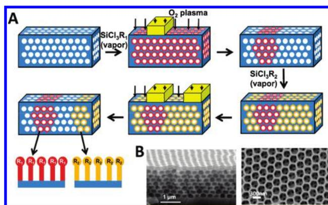
**Figure 1.** (A) Schematic of the chemical encoding procedure. The inner surfaces of IOFs are functionalized by repeated iterations of exposing the entire film to alkylchlorosilane vapors, followed by selective exposure to oxygen plasma, masked through slabs of PDMS, sealed on top of the film. (B) Scanning-electron micrographs of IOFs, left: cross section; right: top view.
