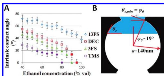
**Figure 3.** (A) Measured contact angles from different ethanol concentrations in water on flat silicon surfaces after exposure to 13FS, DEC, 3FS, TMS vapors. Filled markers indicate that regions of an IOF functionalized with the same groups are being infiltrated by the corresponding EtOH/water mixture. (B) Schematic of a liquid front propagating through a single unit cell of an inverse opal.
